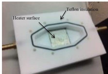
Figure 2. Test section heater (Bayomy et al. 2016)
